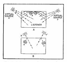
FIG. 3—Reflective speaker system, showing location of virtual sources
