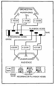
FIG. 2—Block diagram of elements composing three-channel recorder-reproducer
